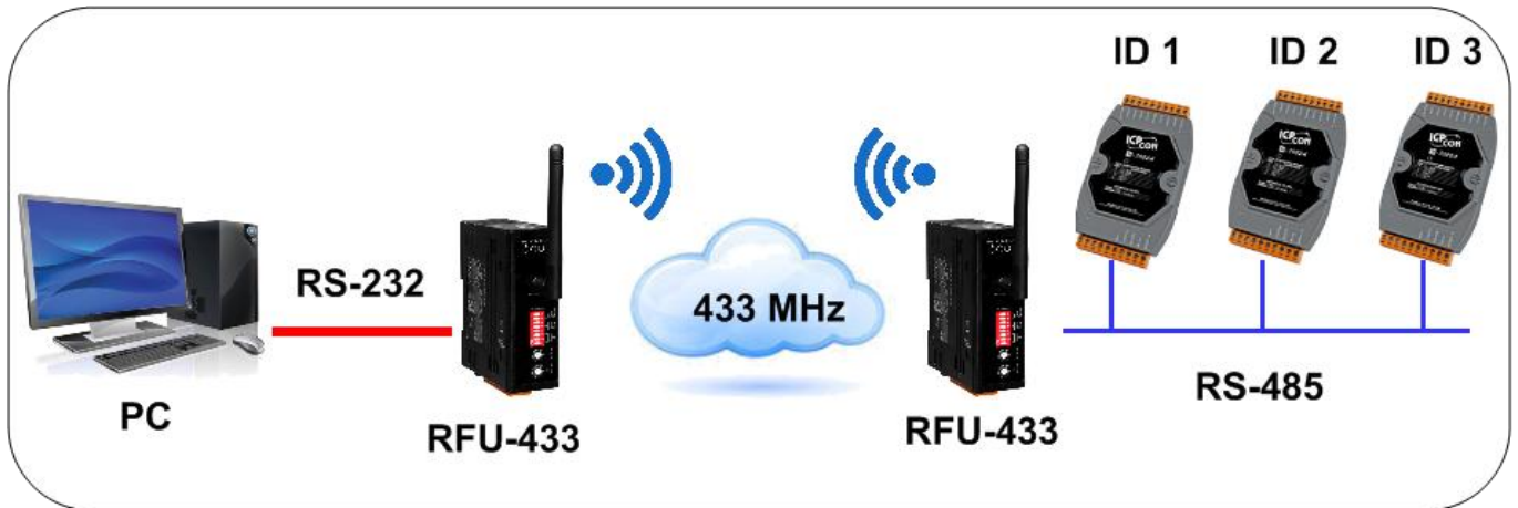
PC controls RS-485 modules 1 ~ 3 through RFU-433.
