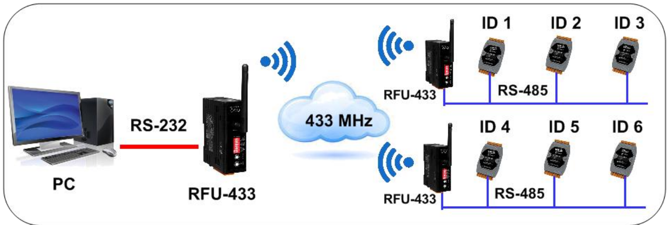
PC controls RS-485 modules 1 ~ 3 through a RFU-433 and modules 4 ~ 6 through another RFU-433
