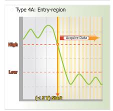
**Pre-trigger Mode:** In pre-trigger mode, the signals are digitized before a trigger condition occurs.
