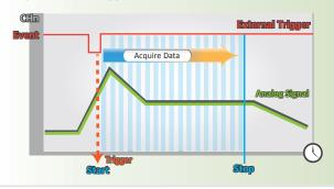
**Middle-trigger Mode:** In middle-trigger mode, the signals are digitized both before and after a trigger condition occurs.
