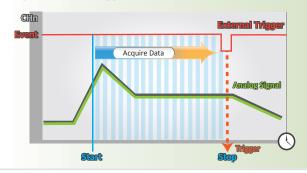
**Delay-trigger Mode:** In delay-trigger mode, signal capture begins once the programmed delay period from the trigger has elapsed.
