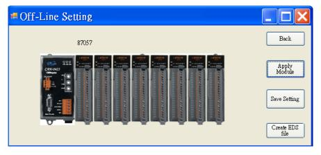
Step 5: Then, repeat the step 3~4 to configure the slot 1 to I-8042 module. Then, click "Save Setting" button to finish the off-line parameter settings.
