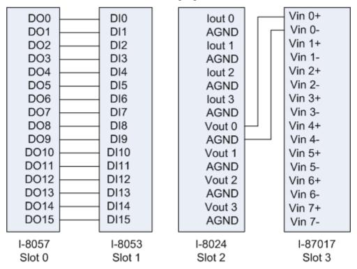
Please use the CAN-8423 rotary switch to set the node ID to 1, and CAN bus baud rate to 125Kbps. Moreover, use CAN Slave Utility to set the I-8024 and I-87017 input/output range to -10V~+10V. When using the CAN Slave Utility, the following information can be as a reference. (Note: CAN-8123/CAN-8223 can't be used with the on-line mode to set the channel input/output range. Therefore, users have to refer to the section 5.5 to know how to use the SDO protocol to set the channel input/output range)
