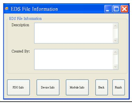
Step 8: Users can select the "PDO Info", the "Device Info" and the "Module Info" button for purpose to view the PDO objects, device profile and slot module configuration information. These information dialogs are shown below.
