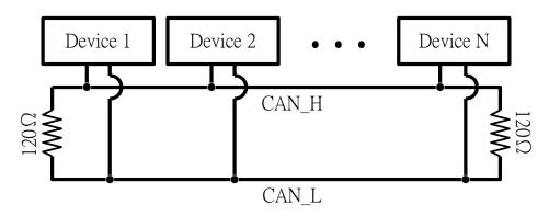
Moreover, to minimize the voltage drop, value of the terminal resistance must be higher than the one defined in the ISO 11898-2. The following table is for users' reference.
