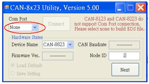
Step 2: Take the CAN slave device (CAN-8823 with node ID 1) as an example, Users have to fill in "NODE ID" with 1 and choose "Device Name" with CAN-8823. Then, press "Next" button.
