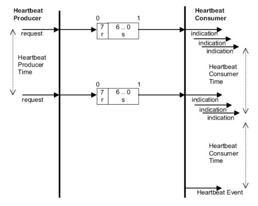
The Heartbeat Protocol defines an Error Control Service without need for remote frames. A Heartbeat Producer transmits a Heartbeat message cyclically. One or more Heartbeat Consumer receive the indication. The relationship between producer and consumer is configurable via the object dictionary. The Heartbeat Consumer guards the reception of the Heartbeat within the Heartbeat Consumer Time. If the Heartbeat is not received within the Heartbeat Consumer Time a Heartbeat Event will be generated.
