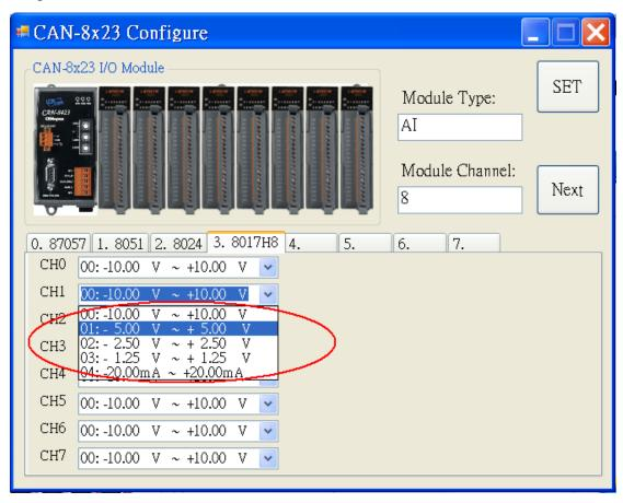
Step 6: After setting the proper output range, users can click "Set" button to store the configuration. If all of slot module configurations are finished, click "Next" button to next step.
