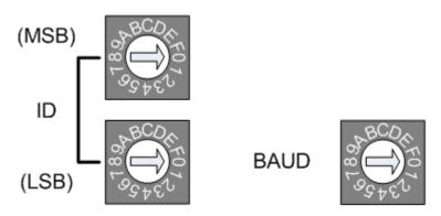
The first two rotary switches (MSB & LSB) control the CAN-8x23 node ID. MSB (Most Significant Bit) means the high nibble of the node ID, and LSB (Least Significant Bit).
