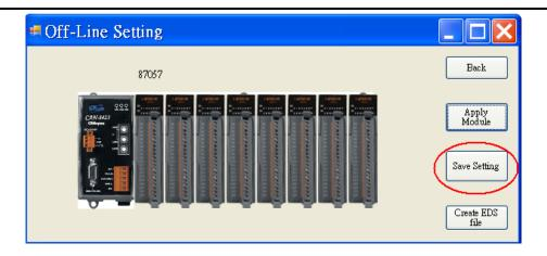
Step 6: Then users can press button "Create EDS Module" for create CANopen slave EDS file.
