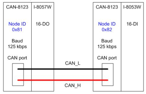
The node ID of left CAN-8123 is "0x81", and the node ID of right CAN-8123 is "0x82". Both of these two module's node ID switch are selected to I/O pair-connection mode node ID, and these two modules will into Operational state automatically. When the DI module, right CAN-8123, receives a DI ON-signal, the DO module, left CAN-8123, will output the ON-signal at the corresponding DO channels.
