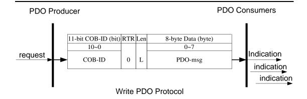
**COB-ID**: the default PDO COB-ID, or the PDO COB-ID can be defined by
