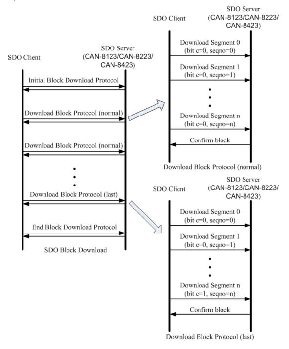
Step 1. When the Initiate SDO Block Download protocol is carried out, the CAN-8423 will be informed with the value of the object entry with index 0x1400 and sub-index 02 modified by the method of the SDO Block Download,
