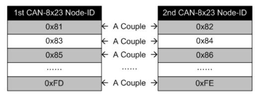
For example, user uses a CAN-8123 with I-8057W and a CAN-8123 with I-8053W to do I/O pair-connection. The connection structure is as follows.
