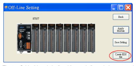
Step 7: The two fields, "description" and "create by", can help users to do some notes in EDS files. If these two fields are empty, the "ICPDAS CANopen I/O Slave Device" and "ICPDAS" will be used as the default value when creating the EDS file.
