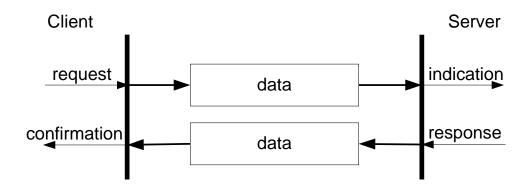
The SDO has two kinds of the COB-IDs, RxSDOs and TxSDOs. They can be viewed in the CANopen device. For example, users send a SDO message to the CAN-8x23 by using RxSDO. On the contrary, the devices CAN-8x23 transmit a SDO message by using TxSDOS.
