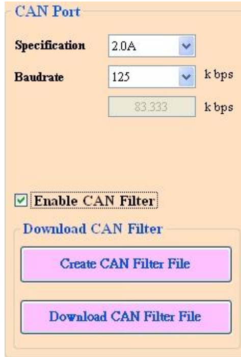
Figure 3-11: The CAN port of I-7530A-MR configuration.
