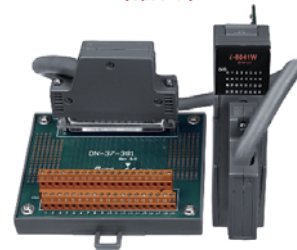
I-8017DW, I-8040W, I-8040PW, I-8041W, I-8041AW, I-8041PW, I-8042W, I-87017DW, I-87024DW, I-87028CDW, I-87040W, I-87040PW, I-87041W, I-87041PW and I-87042W with DN-37-381-A & DB37 Male to Female Cable (Optional)
