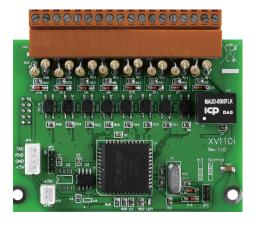
XV110 16-ch Isolated DI (3.5 ~ 50VDC) Expansion Board
