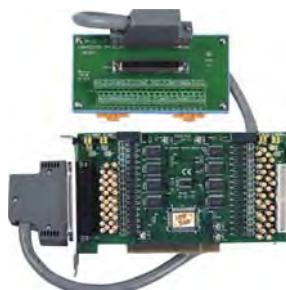
PISO-P64 with DN-37: D-sub 37-pin daughter board with 1 m cable.
