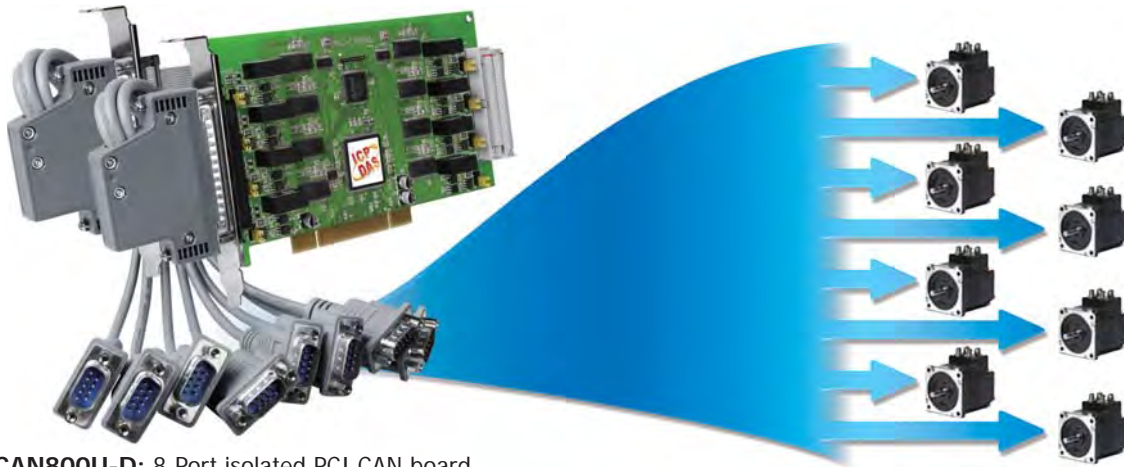
PISO-CAN800U-D: 8-Port isolated PCI CAN board
