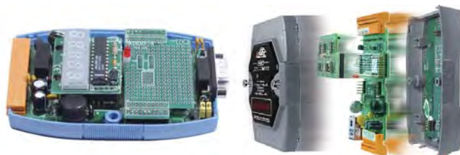
Plug an X-Board into a palm-size PAC
