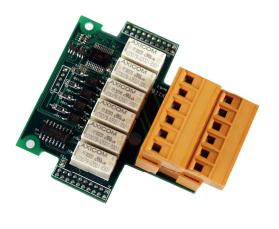
**X116** 6-channel relay output and 4-channel isolated D/I
