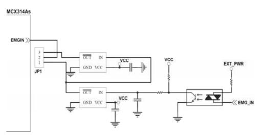
Fig. 2.14 Emergency Stop Signal connection
