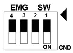
Fig. 1-14 EMG SW setting for user controlled signals.
