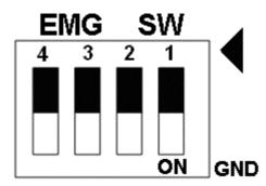
Fig. 2.8 EMG SW setting for user controlled signals.
