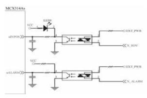
Fig. 2.12 General Digital Input circuit
