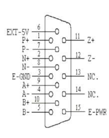
Fig. 3-8 Pin definition for CN5 ~ CN8
