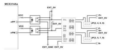
Fig. 2.10 Output pulse example
