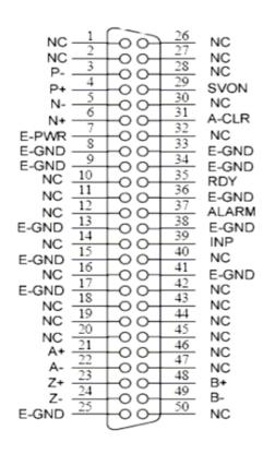
Fig. 1-5 Pin definition for CNX, CNY, CNZ, CNU
