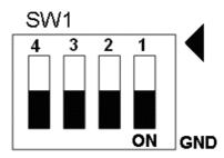
Fig. 3-13 SW1 setting for normally GND (Default setting)
