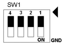
Fig. 3-14 SW1 setting for user controlled signals.
