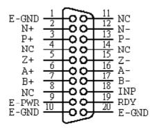
Fig. 1-5 Pin definition for CN-XA,
