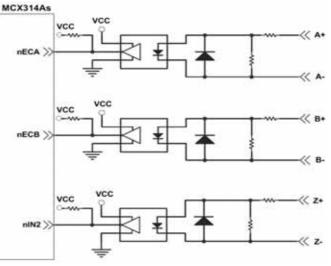
Fig. 2.13 Encoder signal connection
