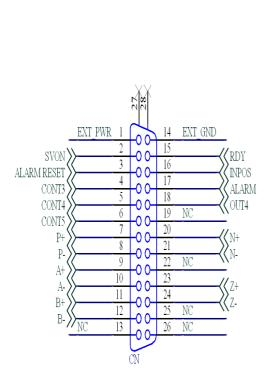
Fig 3-5 Pin definition for CN-X, CN-Y, CN-Z, CN-U
