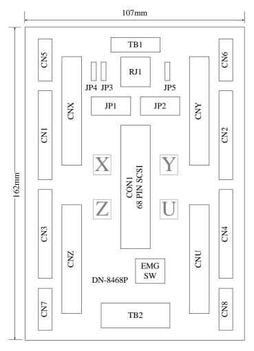
Fig. B2-1 Board layout for the DN-8468P
