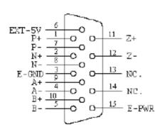
Fig. 3-8 Pin definition for CN5 ~ CN8
