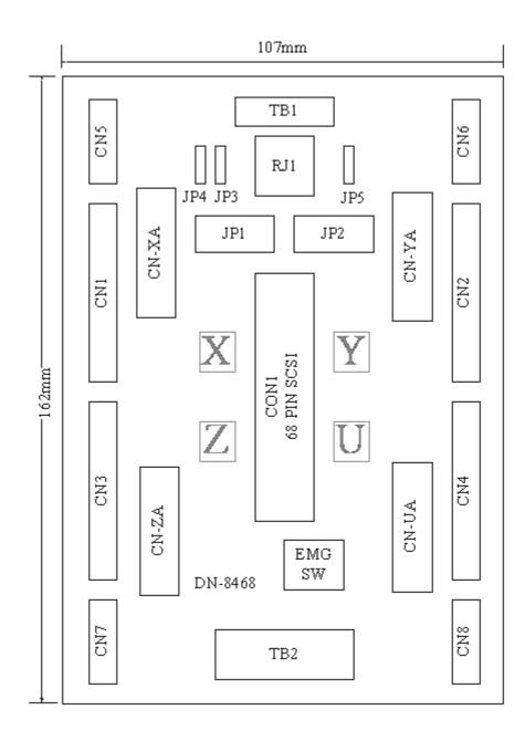
Fig. 3-1 Board layout for the DN-8468FB
