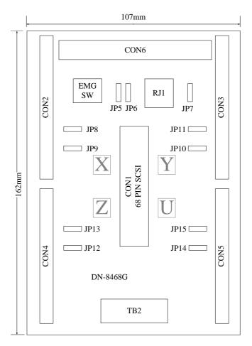
Fig. 2.0 Board layout for the DN-8468G
