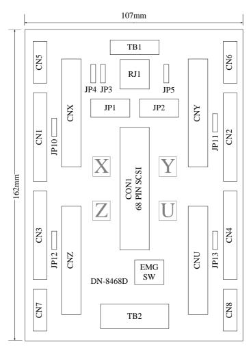
Fig. 3-1 Board layout for the DN-8468D
