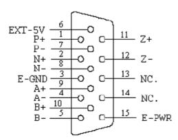
Fig. 1-8 Pin definition for CN5~CN8
