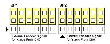
Fig. 3-12 External encoder signals setting
