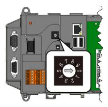
Rotary Switch is an operating mode selector. The XP-8000-CE6 has several operating modes, for more detailed information about these operating mode, please refer to "2.4 Configuring the Boot Mode"
