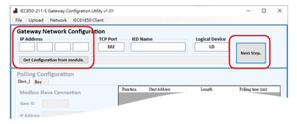
2. If you want to create a new data mapping, please input the Node ID, IP address and port of the Modbus TCP server. And then press "Next step" button.
