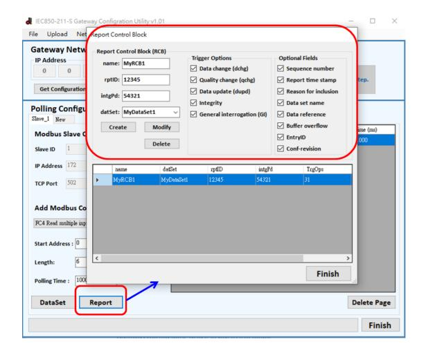
6. Press "Finish" button to convert the configuration to a file named "GatewayConfig.toml" and it is put in the folder "Gateway\_Configuration" which is next to the utility.
