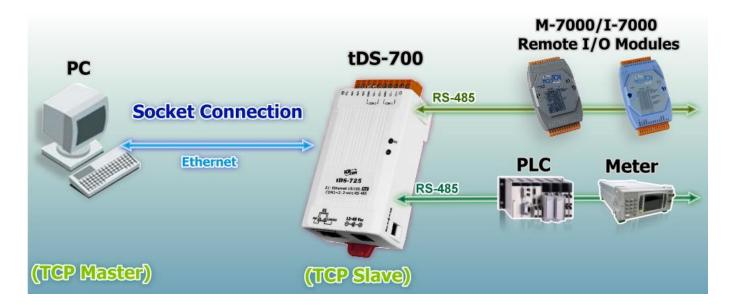
tDS-700/DS-2200 series module can accept the TCP connection (include raw data) directly, it also can communicate with TCP client and Serial Device in this way.
