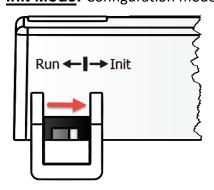
For tDS-700/DS-2200 series modules, the operating mode switch is set to the **Run** position by default. In order to update the firmware for the tDS-700/DS-2200 series module, the switch must be moved from the **Run** position to the **Init** position. The switch must be returned to the **Run** position after the update is complete.
