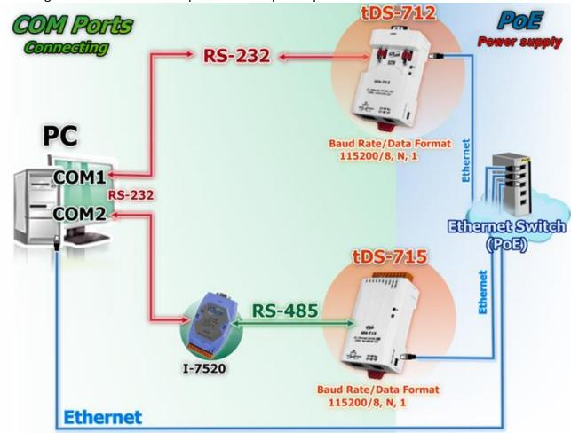
The image below shows an example of the setup for a pair-connection test:
