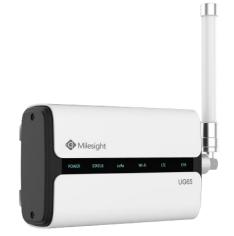
UG65 is a robust 8-channel indoor LoRaWAN<sup>®</sup> hotspot, which is compatible with Helium LongFi technology. Adopting SX1302 LoRa chip, high-performance quad-core CPU and secure crypto chip, UG65 provides high-efficiency and reliable connection. UG65 has line of sight up to 15 km and can cover about 2 km in urbanized environment, which can cover larger areas and provide connectivity to more than 2000 nodes.
