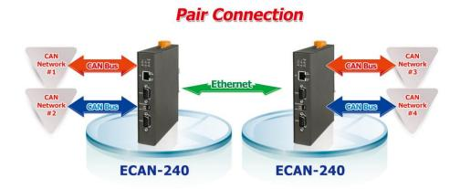
When using the **UDP protocol**, the application architecture will be either one-to-one or one-to-many (UDP broadcast), as illustrated in the application diagram below.
