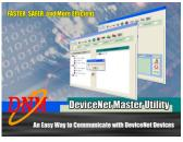
This utility supports to search all devices and specific devices in the network and can configure the I/O connection of the devices by searching devices or manual setting. It can easily to access the I/O data of all the slave devices.
