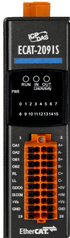
Figure 5: ECAT-2091S front view with motor and encoder in- and outputs
