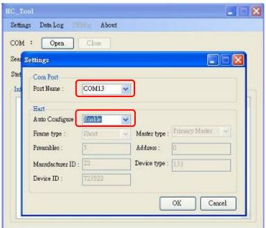
Figure 3-3: Set "Com Port" and "HART" Parameters
