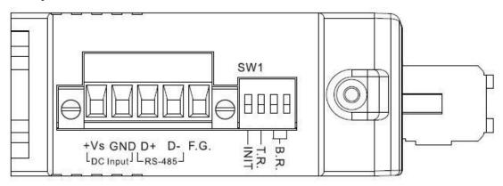
The M-2017 is an 8-channel voltage and current input module, with the ability to connect various types of inputs to a single module. It supports for fast mode, 60 samples/second. The M-2017 modules are designed for industrial plant environments and have special input circuits to provide 240Vrms continuous overload protection.
