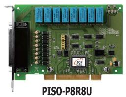
Universal PCI, 8-ch Optically Isolated Digital Input and 8 Relay Output Board
