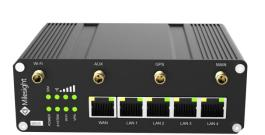
UR35 is a cost-effective industrial cellular router with embedded intelligent features that are designed for multifarious M2M/IoT applications. Global WCDMA and 4G LTE carrier supported make this drop-in connectivity a great help for operators in maximizing uptime.
